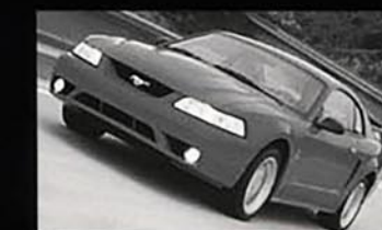
1999 SVT MUSTANG COBRA 320 horsepower 4.6-liter dohc V8 Independent rear suspension introduced Traction control introduced Production: 8,095 units
