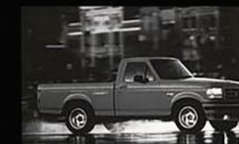
1993-1995 SVT F-150 LIGHTNING 240 horsepower 5.8-liter ohv V8 E40D four-speed automatic transmission Tow rating: 5,000 lbs.; payload: 745 lbs. Production: 11,563 units
